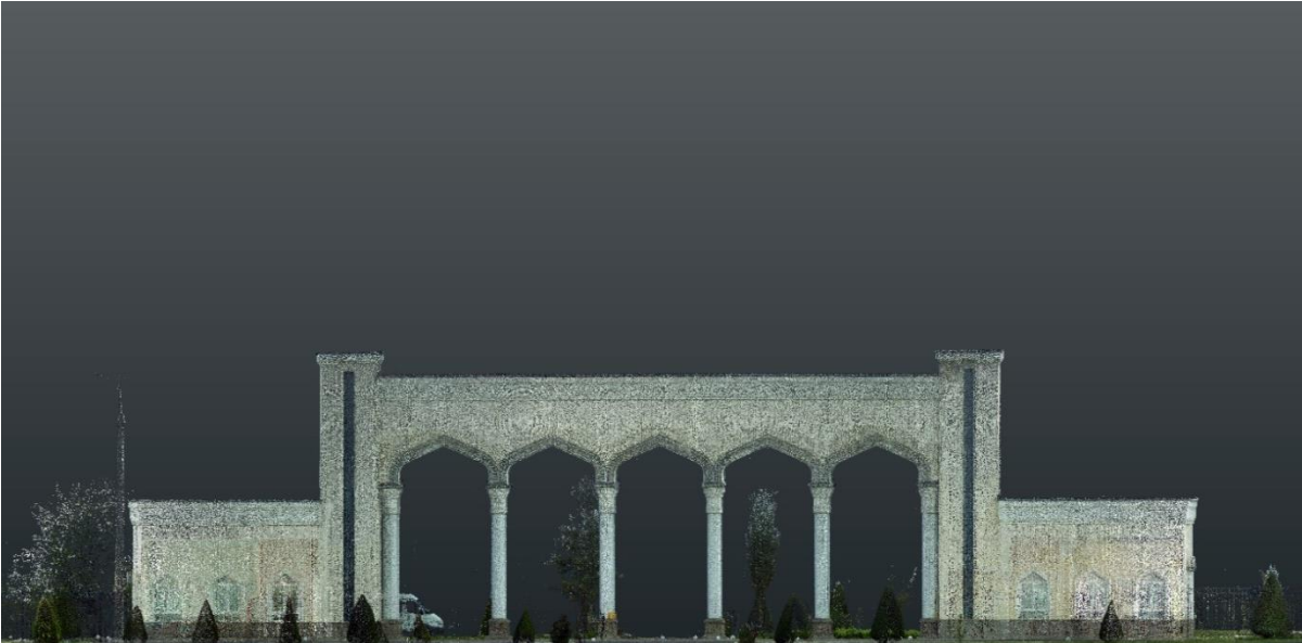
View #3. Front facade of the building, created using 3D results scanning
