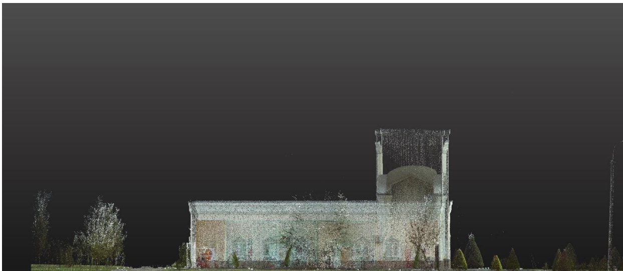
View No. 6. Side facade of the building created using 3D results scanning
