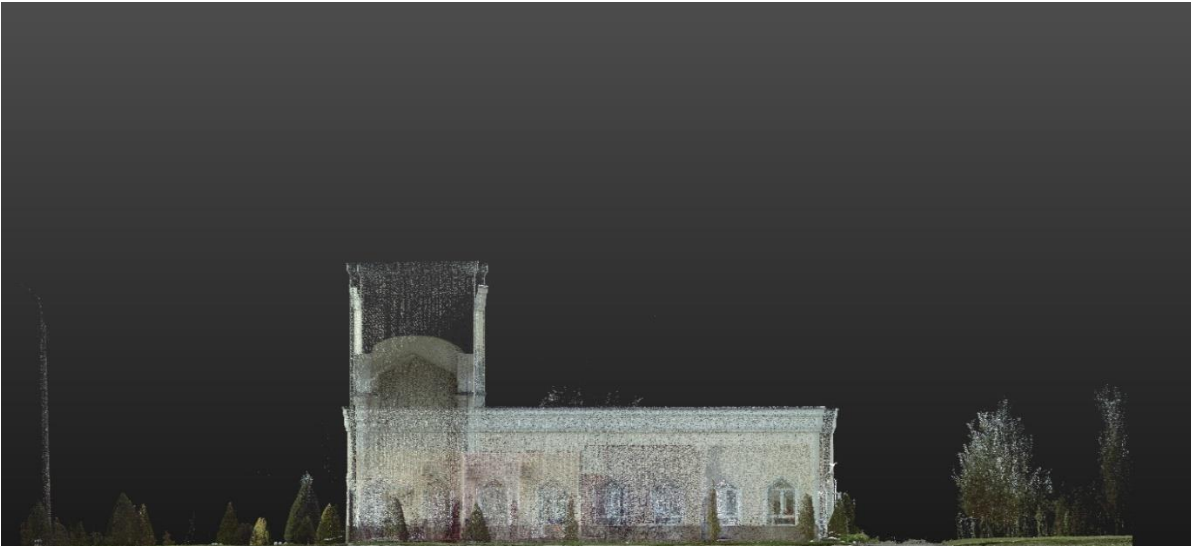
View #4. Side facade of the building, created based on 3D results scanning
