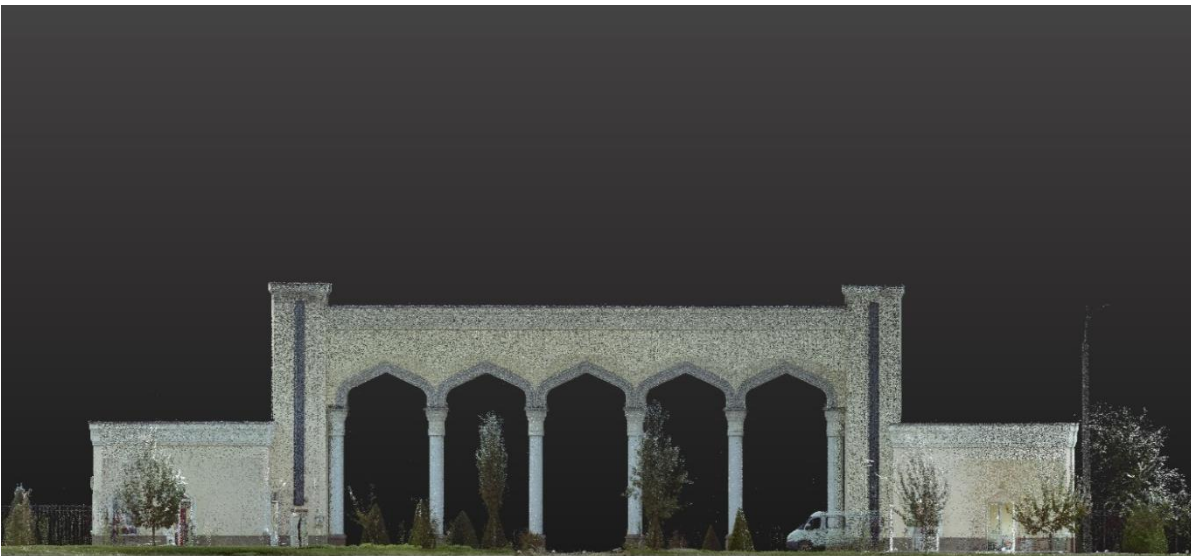
View #5. Rear facade of the building, created using 3D results scanning
